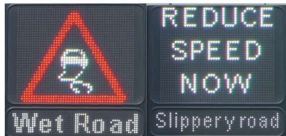
This **sensor-to-sign system**, premiered during TRAFFEX 2003 in Birmingham, is the ideal solution to cover critical microclimatic situations, such as bridges or road sections in lake areas with high risk of unexpected freezing conditions. The quick processing of the sensor data into clearly readable warning messages on the LED VMS allows immediate information to the motorists and thus reduces the risk of road fatalities and injuries.
