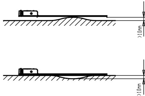
The clearance between the scale and the ground is more than 10 mm. The scale is deformed too much
