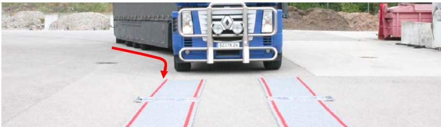
Vehicle not aligned. Rear axles will be outside the scale platform.
