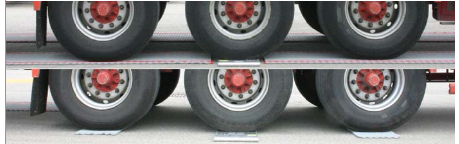
Correct levelling of multiple axle configuration using long or short mats.
