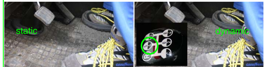
No braking while weighing! Dynamic: 1 st gear and no acceleration!
