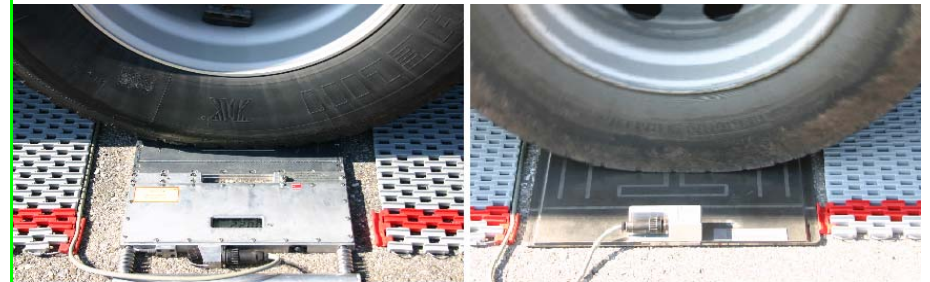
Wheel correctly within the limits of the active weighing area.
